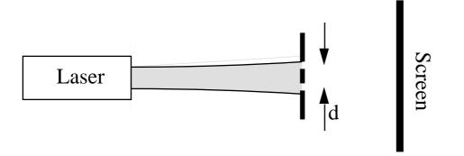
In order to see a high contrast interference pattern on the screen the phase difference between the light at the two slits must be constant. Typically, laser light is found to be spatially coherent across the whole of the beam.
