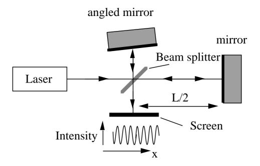
Even when L is large, interference fringes are still observed. This tells us the present phase of the light is strongly related to the past phase.
