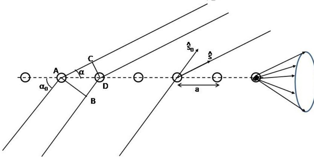
Figure 2: For reinforcement AC-BD should be integer times wavelength,  $\hat{s}_0$  and  $\hat{s}$  are unit vectors in the direction of incident and diffracted beams respectively
