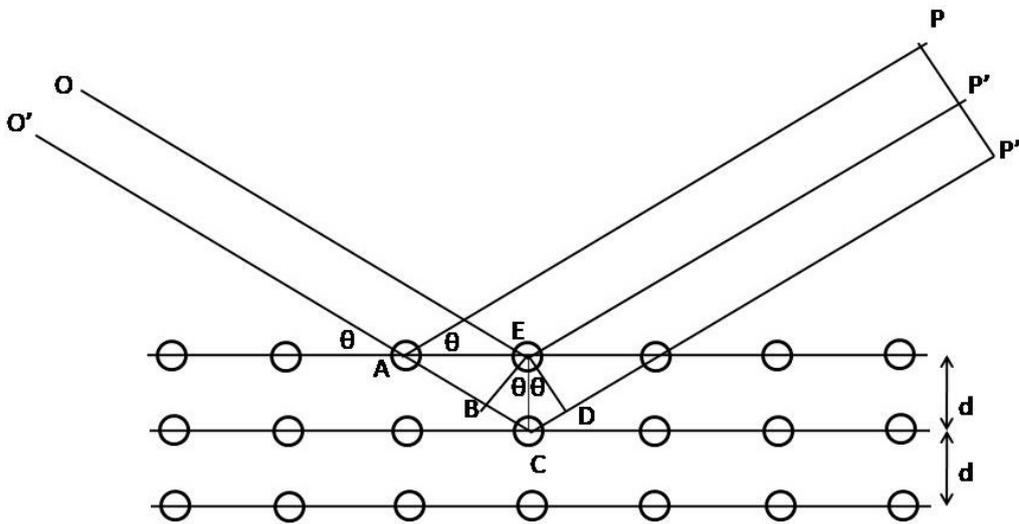
Figure 1: Beams reflected from successive planes interfere constructively only if  $BC+CD$  is an integral multiple of wavelength
