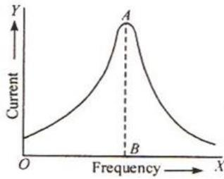
**Resonance.** The variation of current with frequency in an electric circuit containing resistance, inductance and capacitance in series is shown in Fig. 11.8.
